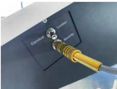
A switch that allows you to use the traction mode cervical or lumbar is placed on the side of the device
