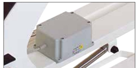
AC0017 AUXILIARY BATTERY Enables the table to be used without power supply. It can be attached to the table by plugging the battery cable directly into the actuator. The battery comes with a support so it can be secured to the frame base. Works for 10 height-adjustment cycles. Power supply: 1.2Ah 24V.
