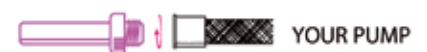
As an alternative to accessory 03111 FASTER BLASTER, it is possible to use a normal bicycle pump by using the included adaptor.
