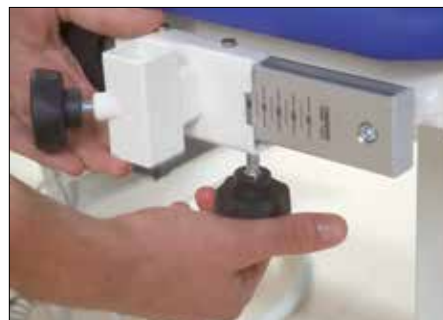
Step 2: positioning by sliding, and fixing the block device
